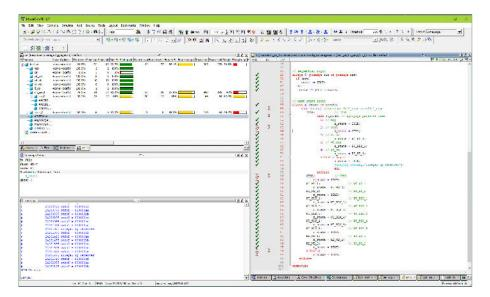
Using integrated code coverage, ModelSim tracks how much of the design has been tested.
