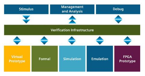
The Siemens EDA Enterprise Verification Platform (EVP) delivers high performance verification from prototype to silicon.
