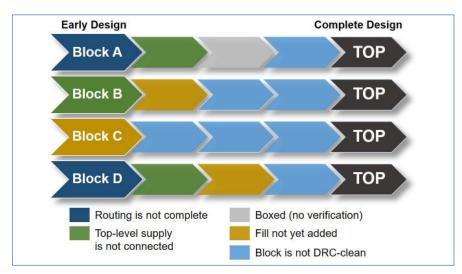
Running targeted verification flows in parallel with block development reduces overall DRC iterations and time.
