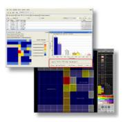
The Calibre nmDRC-Recon DRC Analyze function enables fast, in-depth visualization and analysis during error review and debugging.
