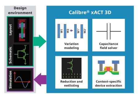
Calibre xACT 3D provides a complete parasitic extraction solution with deterministic field solver accuracy, process variation modeling, electrically aware reduction, and industry-standard netlist formats, all within the design environment.
