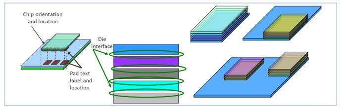
Calibre 3DSTACK uses information supplied in the rule deck to support the various stacking configurations.
