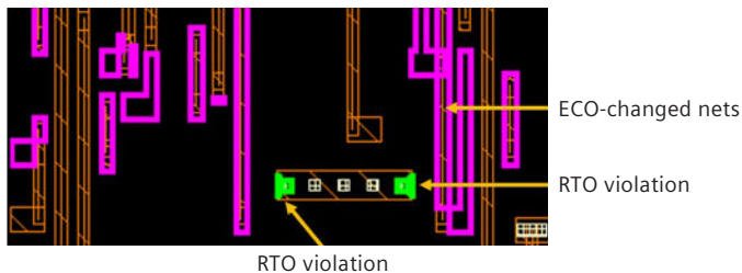
Figure 9: RTO via enclosure error due to ECO change after initial tapeout of specific design layers.
